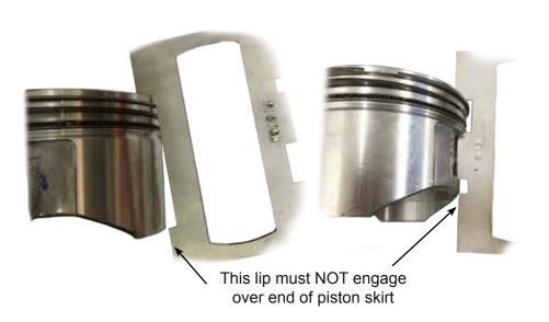
At both sides, this gauge must NOT fit over ends of piston skirt
